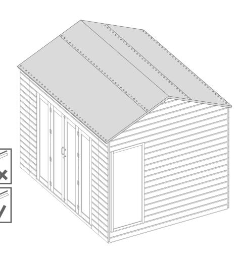
Attach the cover trims each corner of the building and across each joint between the fixed panels, using 3x30mm screws per cover trim.
