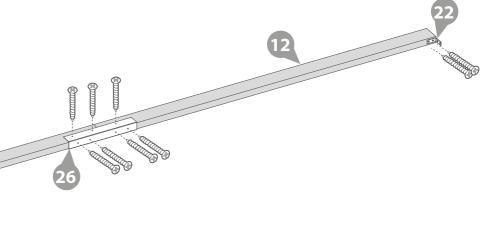
Align the ridge bar between the gables and secure to the central uprights with 2x30mm screws per bracket, as shown in the illustration.
